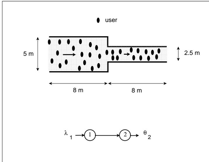
Fig. 5. 2-node system under analysis.
