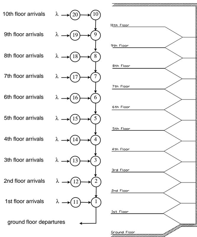
Fig. 9. A 10-story building section and queuing network.
